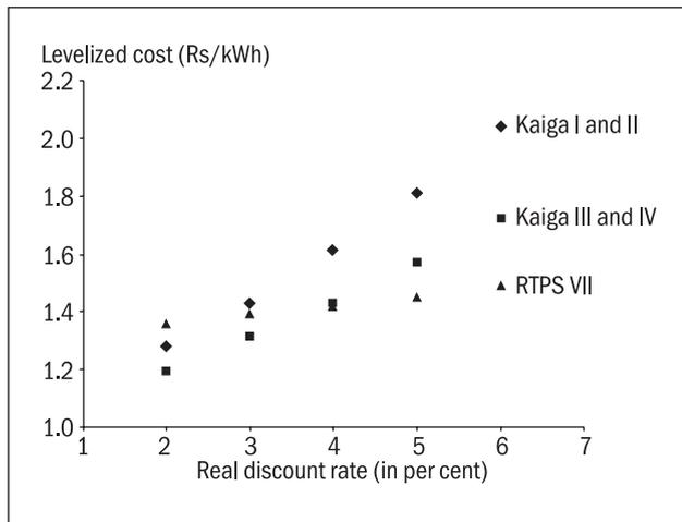
**Figure 1** Levelized cost (the bare generation cost, which does not include other components of electricity tariff like interest payments and transmission and distribution charges) of Kaiga I & II (operating reactors), Kaiga III & IV (reactors under construction; projected costs), and Reichur Thermal Power Station VII (operating thermal plant) as a function of real discount rate<sup>1</sup>
